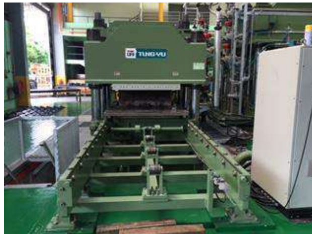
1200 TONS COMPRESSION PRESS 1.2M X 2.2M
