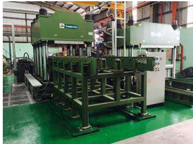
2000 TONS COMPRESSION MACHINE 1.2M X 3.2M
