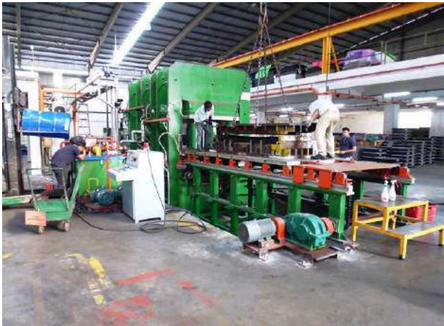
2000 TONS COMPRESSION MACHINE 1.5M X 3.5M
