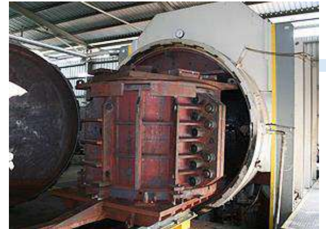
1800 TONS HYDRAULIC BUILT INTO AUTOLAVE FOR CURING
