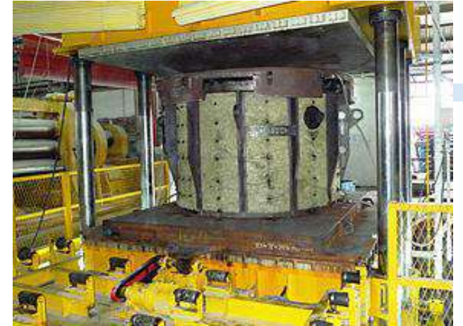
2000 TONS COMPRESSION MACHINE 3.5M X 3.5M X 3M
