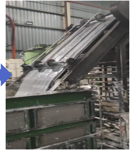
Sheeting process using the two roll mill
