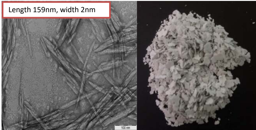
Figure 5: TEM micrograph of cellulose nanocrystal.
